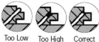
**Note:** Only use flooring nailers that are fully adjustable and that engage the top profile over the tongue at the appropriate angle. Make sure that the flooring nailer is in good working condition and seats properly against the board to prevent top edge and surface dimple damage.
